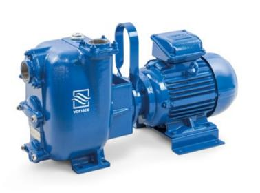
**Product Data** Suction port Threaded - 3" ISO 228 (BSP) Delivery port Threaded - 3" ISO 228 (BSP) Qmax 80 m<sup>3</sup>/h - 1333 l/min (352 USgpm) Hmax 21 m (69 ft) Solids handling 28 mm (1,1 ") Motor power 4 kW - 5,5 HP Motor type **IEC** standard Winding for inverters **Cast iron frame**
